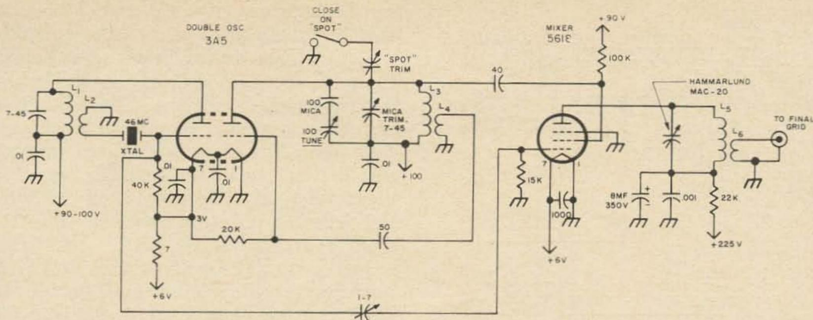
Fig. 2A. Double oscillators and heterodyne mixer.
