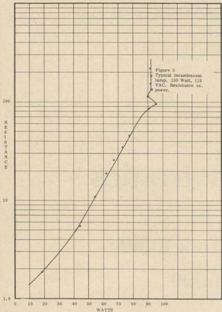
Fig. 5. Resistance versus power input, 150 watt lamp.
