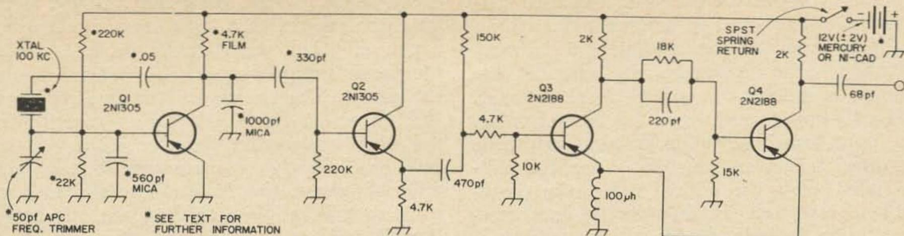
Fig. 1. Schematic of the modern 100 kc calibrator.
