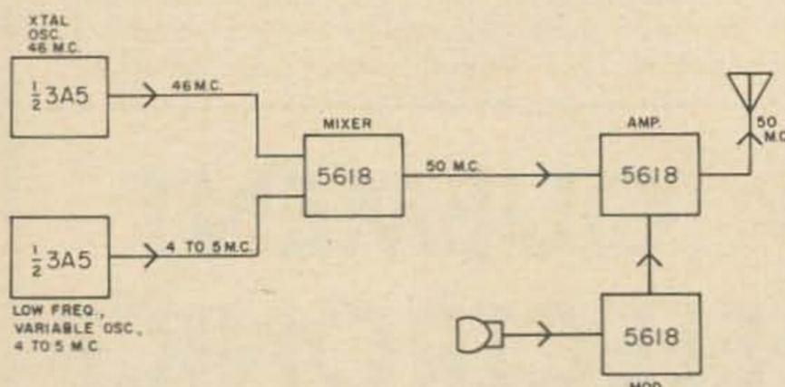
Fig. 1. Block diagrams of heterodyne rig.
