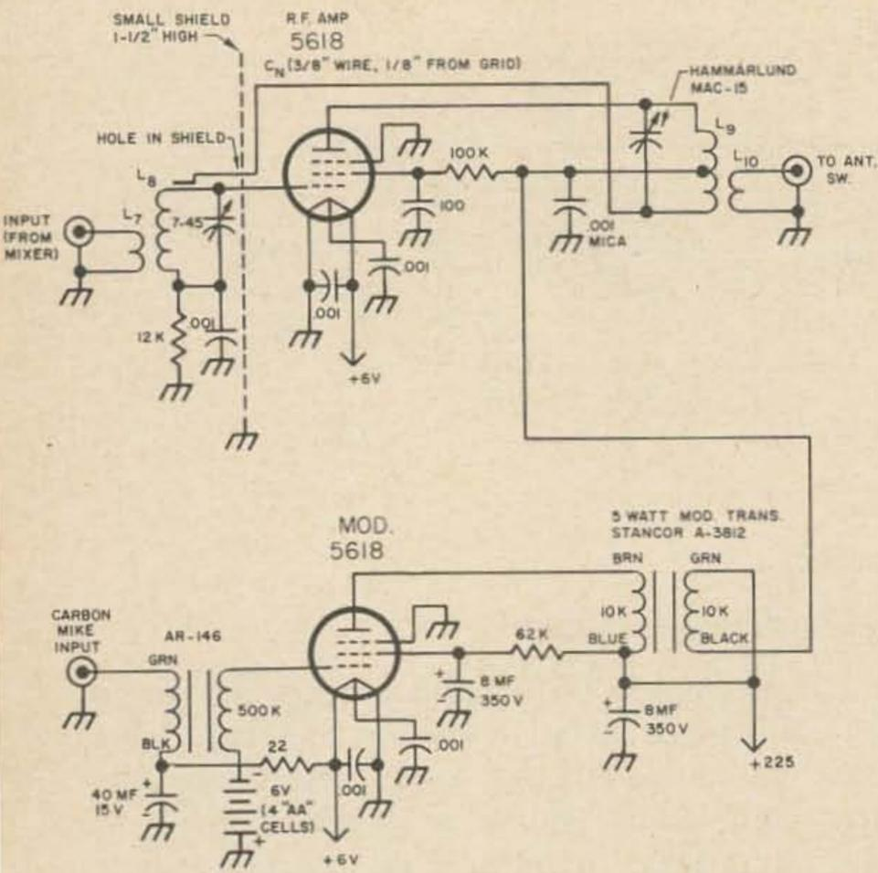
Fig. 2B. RF final and modulator.
