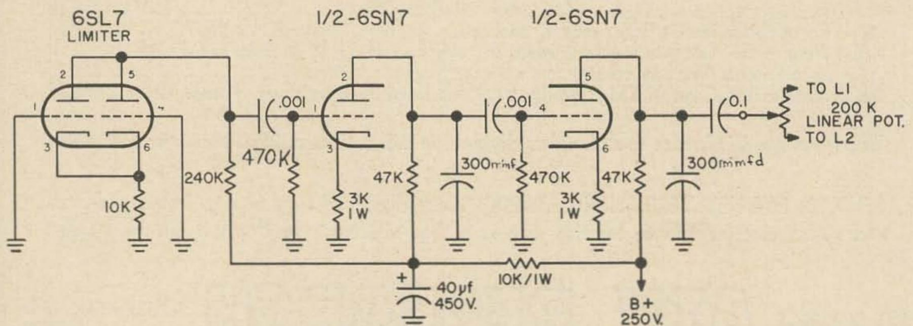
A 12AU7 could be used in place of the 6SN7.
