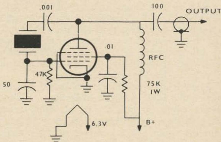
to it. As a bonus, you can plug the unit into your receiver accessory socket and use it as a band-edge marker, with a 3.5 mc crystal.
