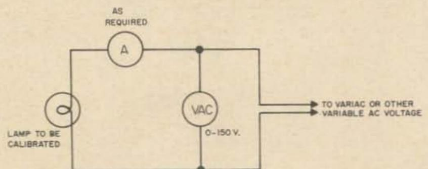
Fig. 2. Method of calibrating lamp and determining resistance.
