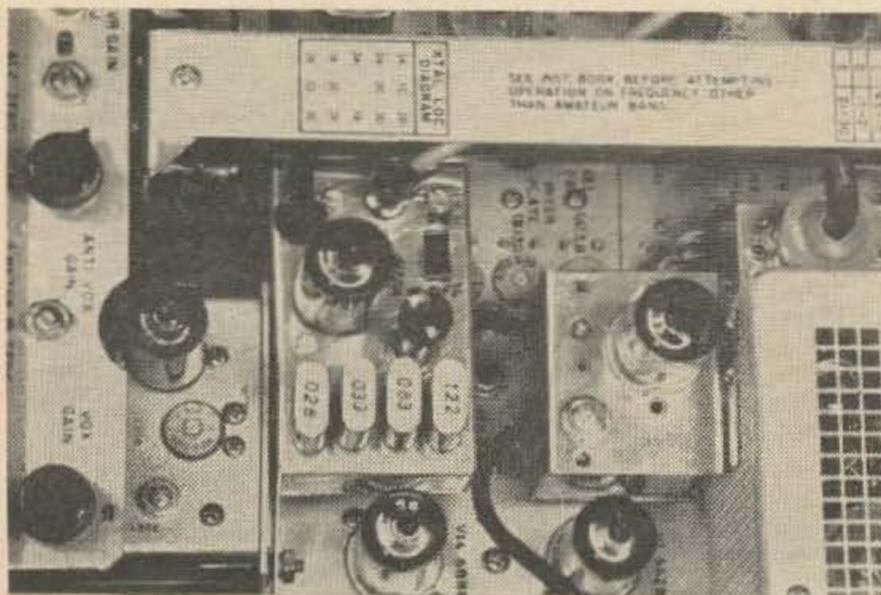
Adapter installed in KWM-2.
