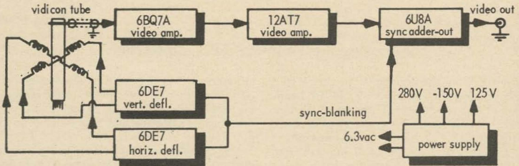
The camera requires 6 hard-to-find components. They are: (1) focus-deflection coils, (2) power transformer (125vac @100ma & 6.3vac @3 amp), (3) vidicon tube socket, (4) 25mm lens, (5) lens mount, (6) small coils kit (two 4-30mh adj coils and five video peaking coils—36uh, 76uh, 96uh, 180uh & 350uh). With this information, make your kit selection on the basis of the parts you need.
