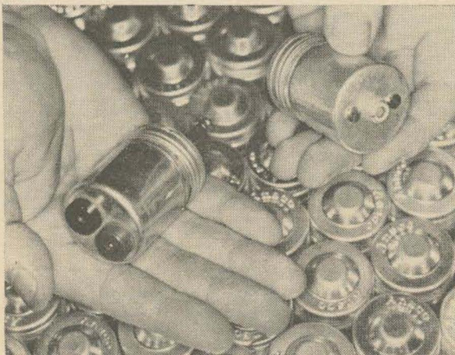
Various handy plug and socket adapters may be made from discarded 35mm film cans. These are made of soft aluminum and will readily accommodate many different types and sizes of plug to socket (and vice versa) arrangements to suit your particular needs. Two configurations which I found valuable in my shack are shown in the photo.
