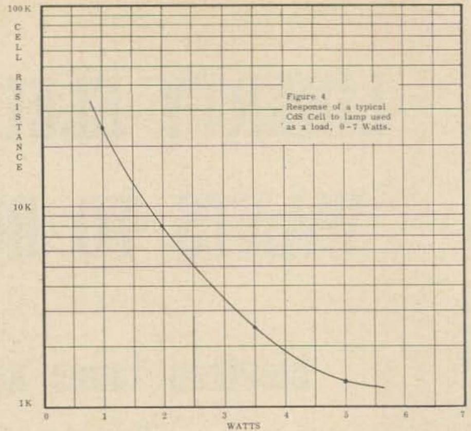
Fig. 4. Response of cell to 7 watt lamp.
