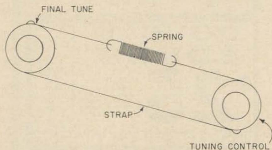
The Heath Apache, a very fine rig, has one undesirable feature: backlash in the "Final" tuning control.
