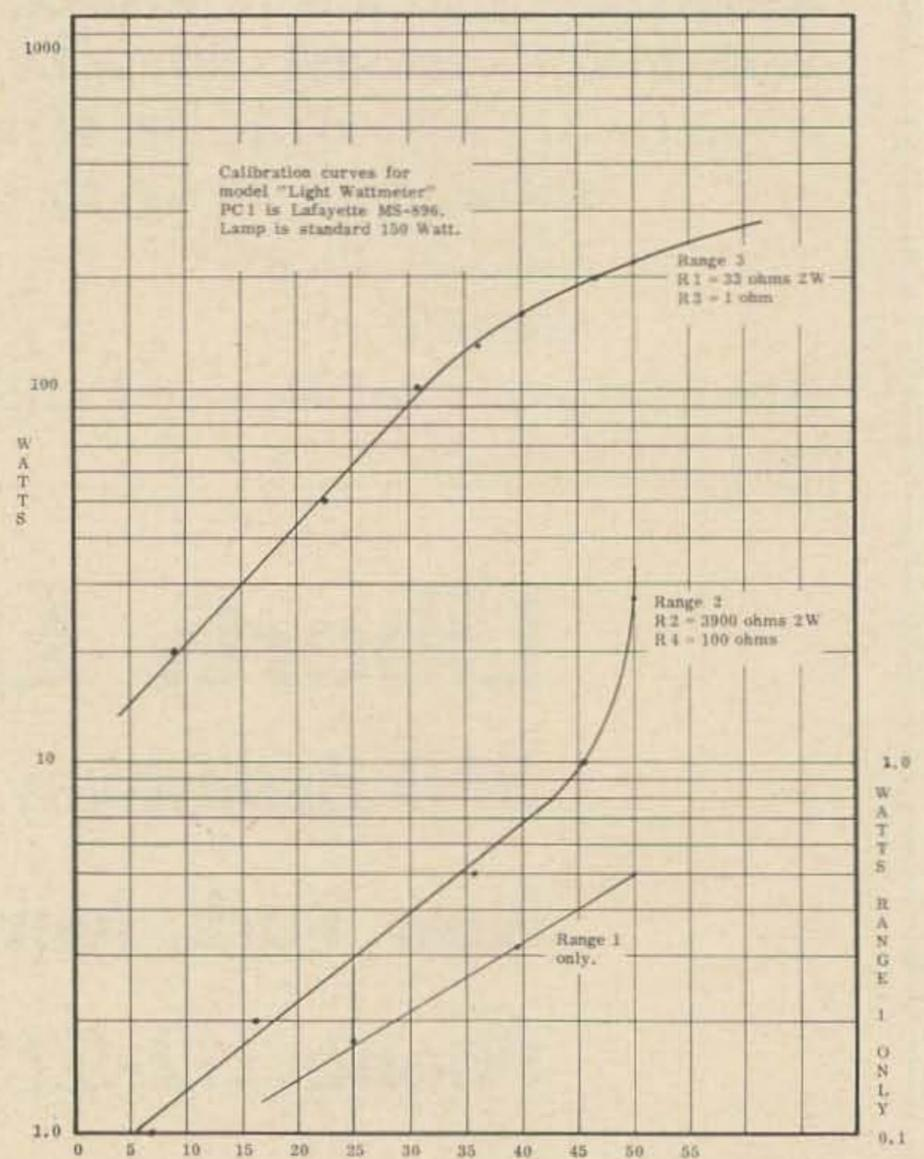
Fig. 6. Calibration curve for Light Wattmeter.
