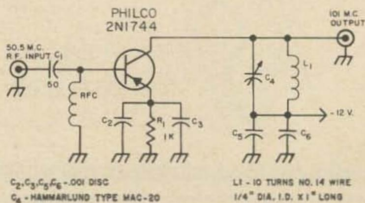
Above is Fig. 2, connections for the transistors used. To the right is Fig. 3, the first doubler.
