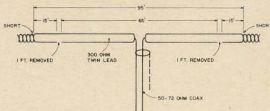
twin-lead a half wave dipole for 40 meters.
