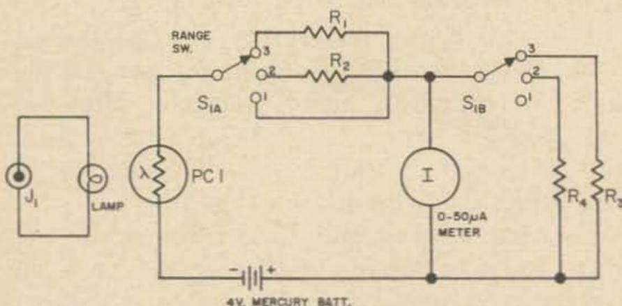
Fig. 1. Circuit of Light Wattmeter.
