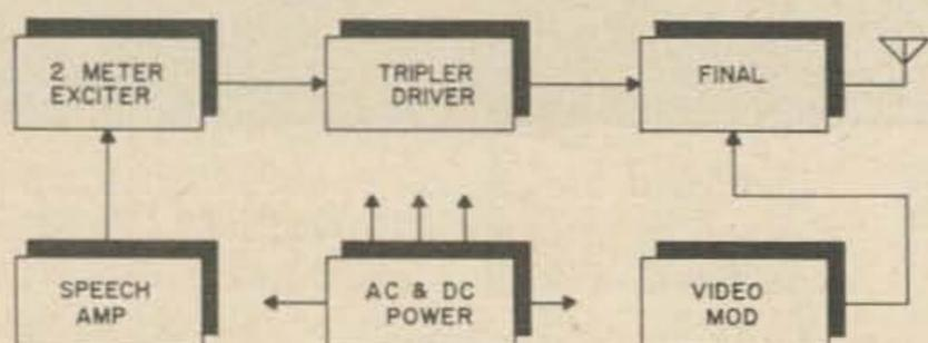
Fig. 1. Block diagram of the ATV-audio transmitter.
